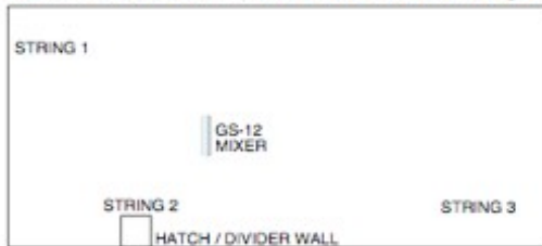
Underground Tank Rectangular, Underground, Concrete 2.5 MG Basin, 115ft X 85ft X 20ft Height
