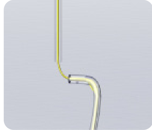
Figure 9: Step 4 & 5 Cut and remove Exterior hose from heating element.
