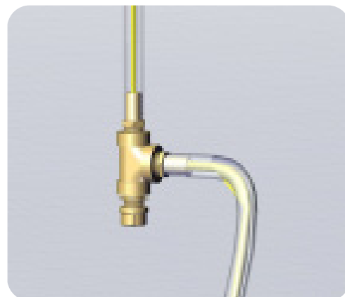
Figure 11: Step 7 & 8 Attach Interior Hose to Penetration Assembly
