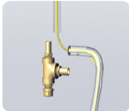
Figure 10: Step 6, 7 & 8 Attach Exterior Hose to Drain Assembly
