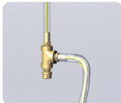
Figure 11: Step 7 & 8 Attach Interior Hose to Penetration Assembly
