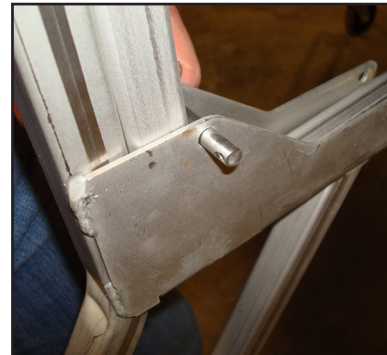
Attaching Leg Extension With a Clevis Pin
