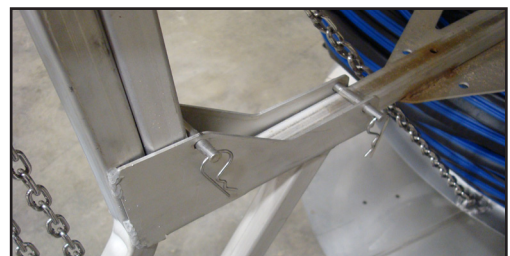
Secured with Hair Pins
