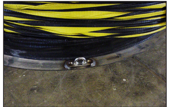
Weld link on hose flange connecting opposite end of chain to hose flange.
