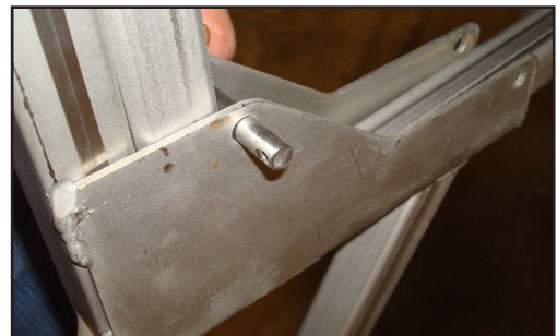
Attaching Leg Extension With a Clevis Pin
