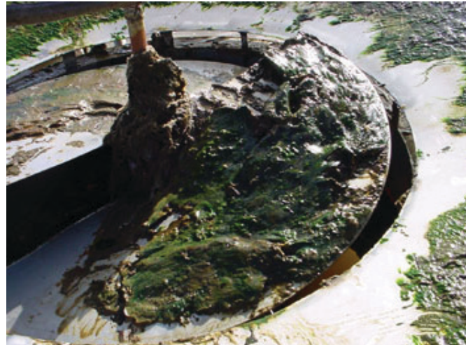
Machine With Buildup On Impeller
