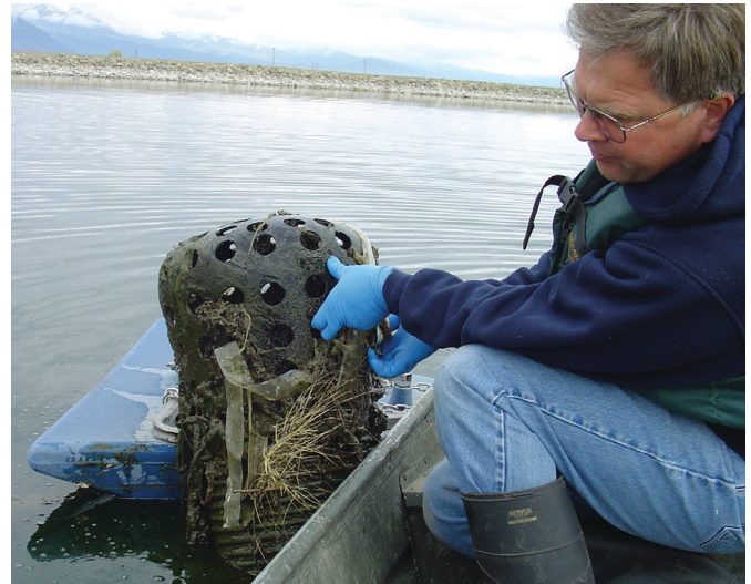
Partially Plugged Strainer
