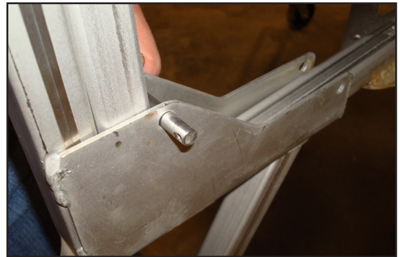
Attaching Leg Extension With a Clevis Pin.
