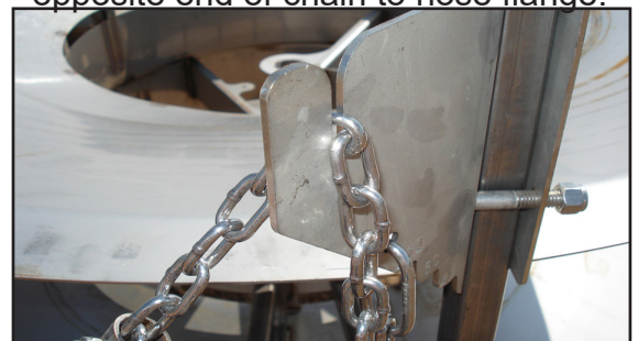
Marker chain slipped into chain bracket slot.
