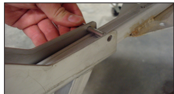
Securing Clevis Pins
