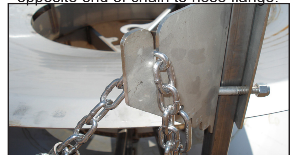
Marker chain slipped into chain bracket slot.
