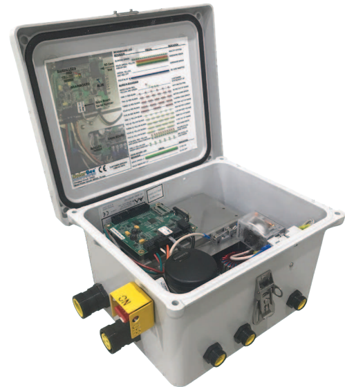
Figure 2: SB B-Series Control Panel, Internal
