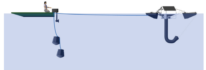
Mooring Blocks Suspended, Ready To Move
