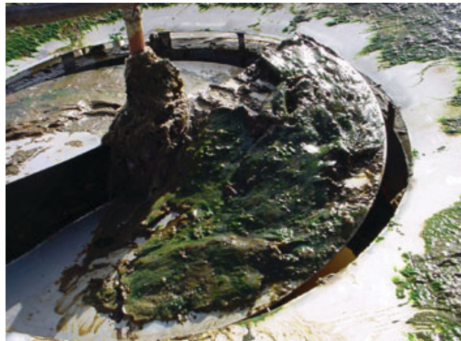
Machine With Buildup On Impeller
