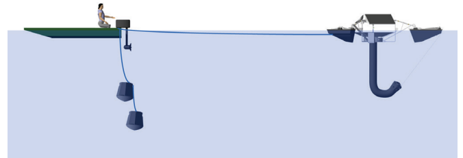
Mooring Blocks Suspended, Ready To Move
