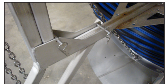
Secured with Hair pins
