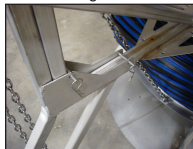
Secured with Hair pins
