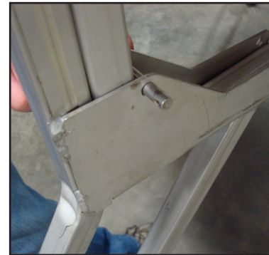
Sliding Leg Extension Around Bottom Leg Of Core Unit
