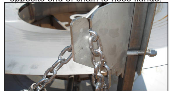
Marker chain slipped into chain bracket slot.
