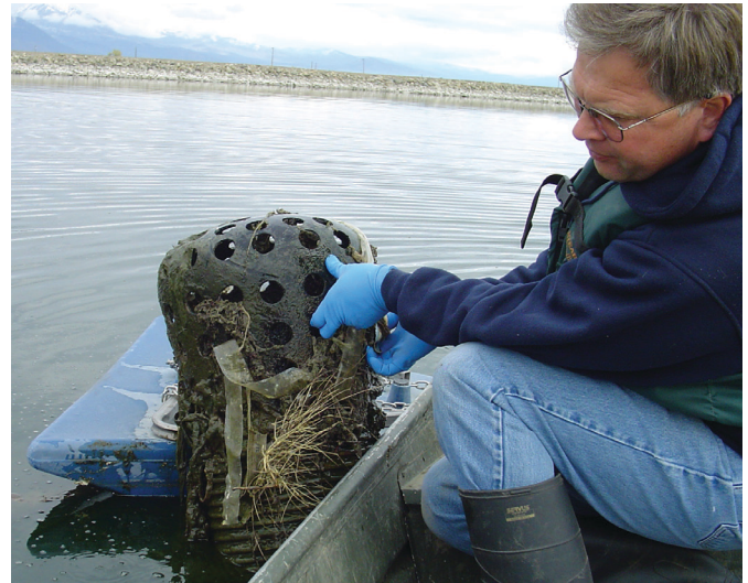
Partially Plugged Strainer
