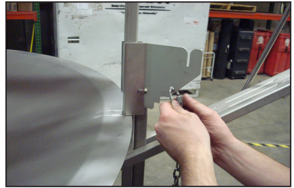
Quick Link connecting end of chain to small chain bracket hole.
