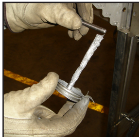
Applying Anti-Seize To The Bolts
