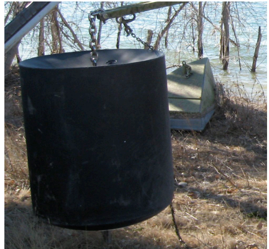
Float upside down chain end toward float arm
