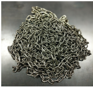
10' T316SS Chain (Retrieval Chain) plus 5 - 1' lengths)
