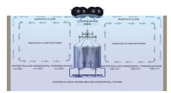
Figure 2: AP Unit Floating Configuration Flow Pattern
