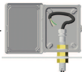
Junction Box & Tank Penetration
