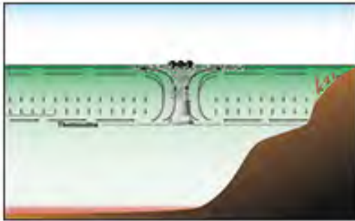
Epilimnetic Circulation for Algae Control In Lakes
