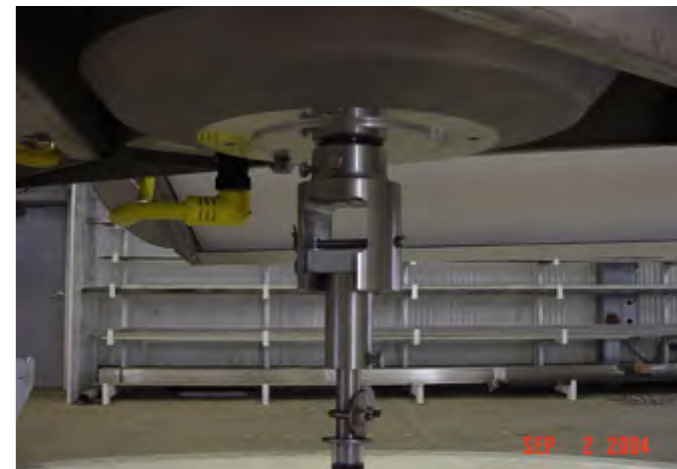
Brushless direct-drive motor (no gear box) provides low-power operation and a 25-year life expectancy
