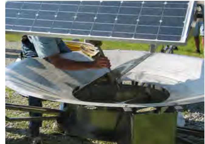
Distribution dish makes the near-laminar flow possible.
