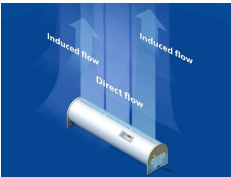
The sheet-flow mixer pulls direct flow into the end of the machine and discharges through 3 long slots on the top of the machine. Direct flow leaves the mixer as a "sheet" of water while also dragging induced flow water up from the bottom of the tank.
